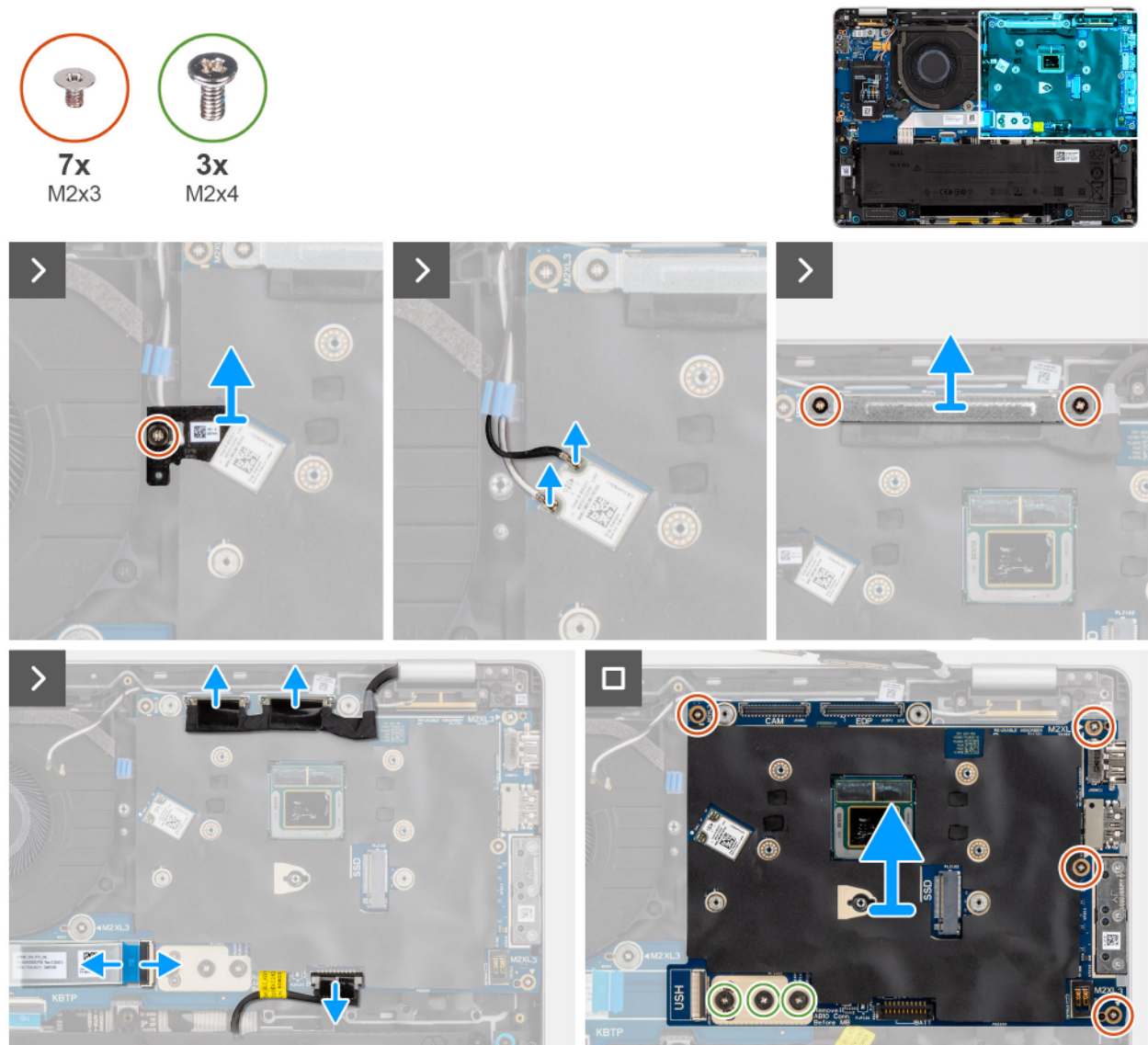
Figure 70. Removing the system board
