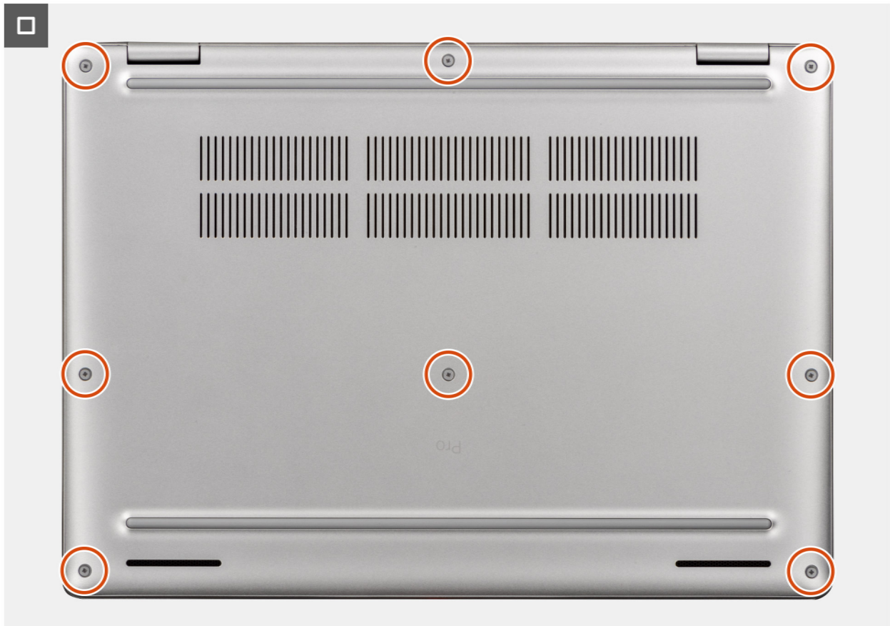
Figure 23. Installing the base cover
