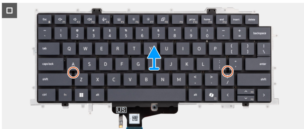
Figure 80. Removing the keyboard
