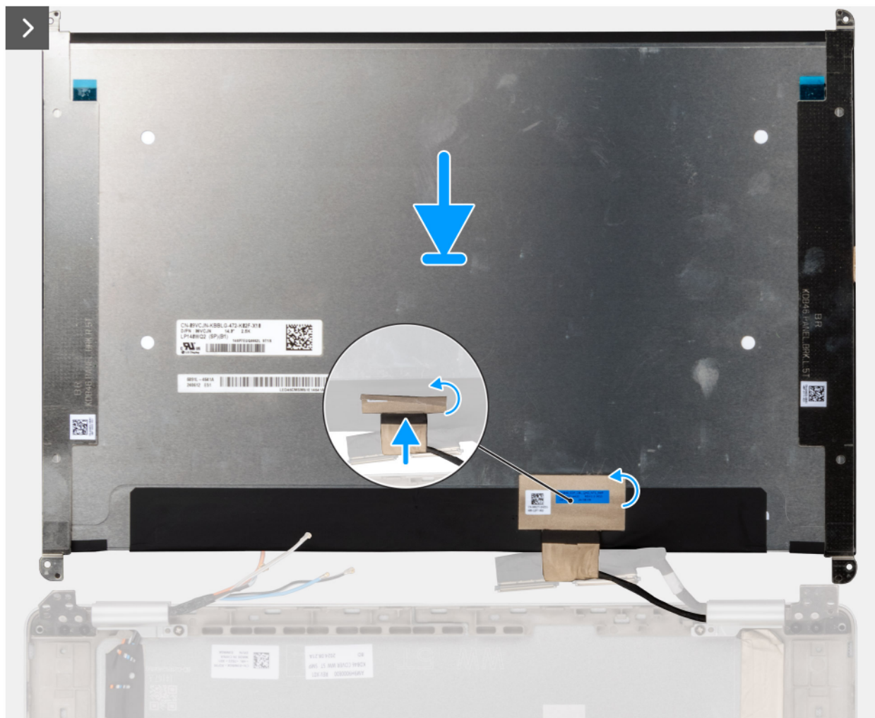
Figure 52. Installing the display cable
