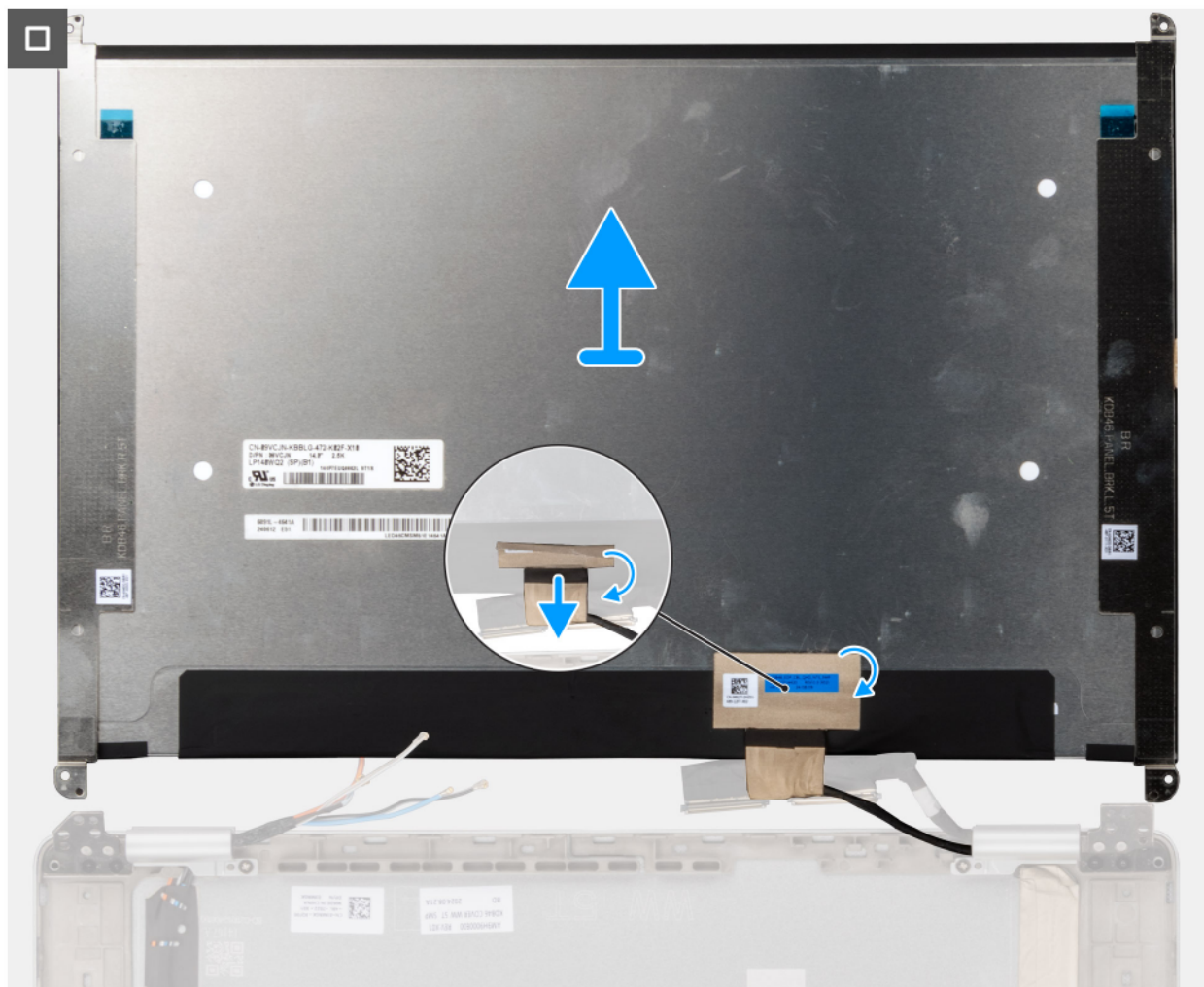
Figure 50. Removing the display cable from back cover
