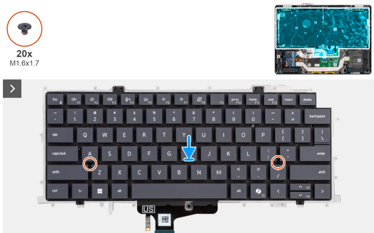
Figure 81. Installing the keyboard
